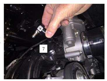
8. Install the retaining clip provided to secure the boost reference adapter in position
