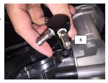
Once installed, the boost reference adapter should look as shown. Vacuum hoses can now be connected.
