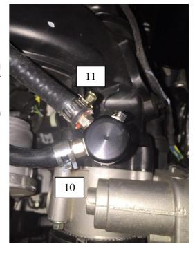
12. Install other end of 1/4" re-inforced hose over barbed end of PCV check valve as shown. No clamp is needed.
